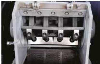
The cutting chamber sits in a soundproofed enclosure to ensure quiet inline operation. The rotor and screen area are easily accessible without for cleaning and maintenance.
