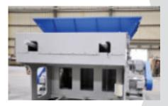
The heavy dutty hydraulic system allows processing of a veriety of materials. The angled hydraulic pusher uses roller guides to avoid blocking and excessive wear.
