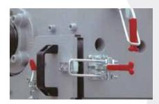
The ZERMA Quick Snap System allows thelower front plate section to be easily removed for granulator cleaning. The lower front plate section is held in position by two sturdy lever clamps.
