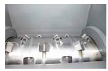
All ZERMA shredders are equipped with our E-style flat rotor. The knives are fixed in special knife holders fitted in machined pockets.
