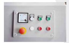
To minimize the needed floor space and make the machine easy to move, machine controls and electrical cabinet are integrated into the machines soundproof housing.
