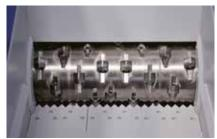
The rotors are equipped with square knives, producing high quality output. The cutters can be turned after they are worn.
