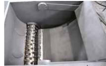
The internal ram design on the ZIS series allows the cutting chamber volume to be increased while keeping a small footprint. Making the ZIS ideal for shredding of big volume parts.
