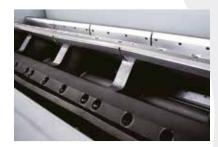
The GSH 1100 series comes standard with wide H-style rotors available with 9,11 or 13 rows of rotor blades ensuring a high quality output.
