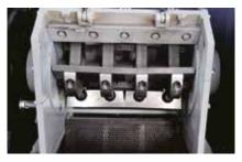
The cutting chamber sits in a soundproofed enclosure to ensure quiet inline operation. The rotor and screen area are easily accesible without for cleaning and maintenance.
