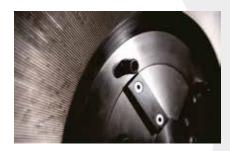
The ZERMA PM Pulverizers can be equipped with either one piece or segmented grinding discs, both are made from high quality tool steel and can be treated to withstand wear longer.
