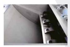
The tangential cutting chamber paired with the aggres sive open rotor design ensures reliable ingestion of voluminous parts. The curved cutting chamber backwall reduces the risk of parts getting stuck.
