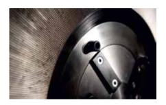
The ZERMA PM Pulverizers can be equipped with either one piece or segmented grinding discs. Both are made from high quality tool steel and can be treated to withstand wear longer.
