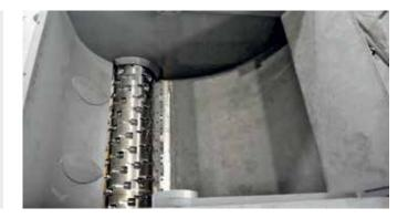
The ZSS / ZPS and ZXS shredders benefit from the sturdy swing ram. The design works without the need for guide rails avoiding the risk of clogging and wear. Two powerful hydraulic cylinders combined with the serrated ram plate ensure a secure grip and good ingestion on all materials. The internal ram design on the ZIS series allows the cutting chamber volume to be increased while keeping a small footprint. This makes the ZIS ideal for shredding big volume parts.
