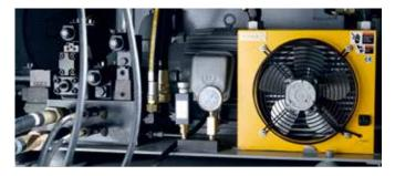
All shredders are equipped with a powerful two speed hydraulic system. This system ensures maximum pressure when feeding material into the rotor and high speeds on the backstroke and running under low load.
