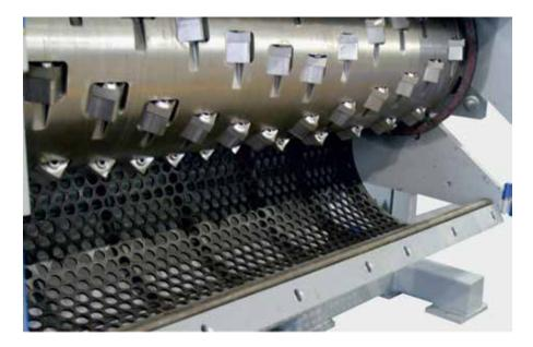
All shredders are equipped with a flat E-style rotor featuring machined pockets for the bolt-in knife holders and knives. The hydraulically lowered screen cradle ensures easy knife maintenance and screen changes.
