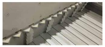
All ZERMA single shaft shredders are equipped with a serrated plate at the front of the hydraulic pusher. This helps ensure constant feeding of the material into the rotor with a variety of materials.
