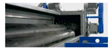
The ZRS pipe shredders are equipped with a special feeding trough sized to take pipes up to 6 m length. A powerful hydraulic ram forces the pipes into the rotor.
