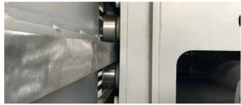
The hydraulic rams in the ZHS and ZRS series shredders are guided by steel rails and large oversized steel rollers. This ensures dependable performance reduced risk of jams and low wear.
