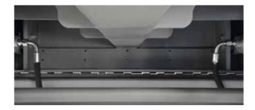
For the processing of thin or fibrous material the segmented floor and pusher on the ZHS series shredders can prevent material from getting lodged under the hydraulic ram, avoiding jams and excessive wear.
